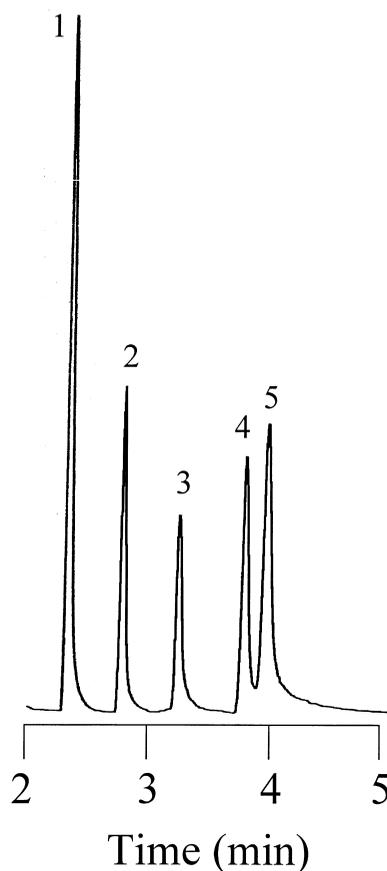
Fig. 3. SGC separation of a standard explosives mixture. Conditions as in Fig. 2. Injected amounts: 0.33 μg NG, 3.3 μg all others. Peaks: (1) nitroglycerine, (2) 2,6-dinitrotoluene, (3) 2,4-dinitrotoluene, (4) 2,4,6-trinitrotoluene, (5) pentaerythritol tetranitrate (PETN).
