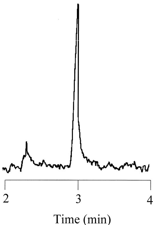
Fig. 2. SGC chromatogram of NG contained in soil sample 1A (*S/N*~90:1). Conditions: 65 cm×320 μm I.D. column packed with ODS-bonded porous (10 μm, 80 Å) particles, neat CO<sub>2</sub> mobile phase, 250 atm, 130°C isothermal oven, 740°C pyrolyzer, 250°C transfer line, 200 nl injection, 12:1 split ratio.
