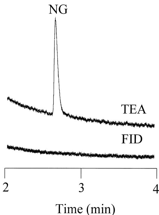
Fig. 4. Chromatograms of standard NG obtained using TEA and FID ( $0.0004 \text{ mg ml}^{-1}$ ). Conditions as in Fig. 3.
